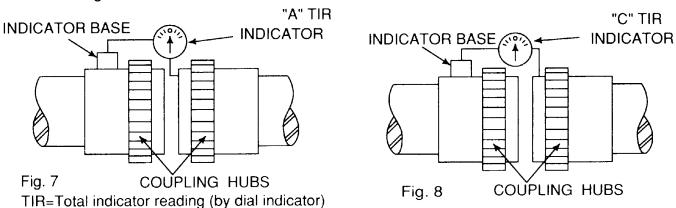
Parallel misalignment is the amount by which the centerlines of the driver and driven shafts are out of parallel. It can be measured using a dial indicator set up as shown in Fig. 8. Again, the couplings are rotated together through 360 degrees so that the indicator does not measure runout of the coupling hub outside diameter.
