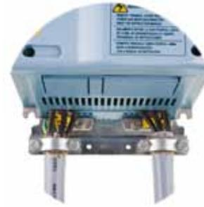
Note: 1) The kit for power cable shielding PCSA-01, PCSE-01 is provided along with VSDs having factory fitted RFI filter.
